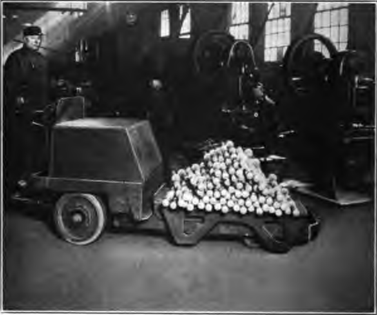
FIG. 4.—4,000-LB. LIFT TRUCK WITH PORTABLE PLATFORM AND LOAD
